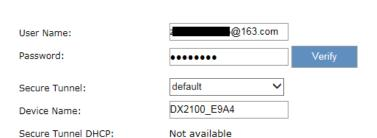
When DHCP server in the secure tunnel network is not available, the IP address of the secure tunnel will be the LAN IP,
